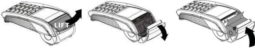
Hold the terminal securely in one hand. With the other hand, and by using two fingers, lift the printer cover release as shown. Fully open the printer cover and remove the old roll of paper.
