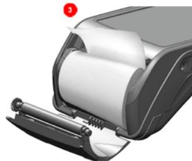
Hold the terminal securely in one hand. With the other hand, and by using two fingers, lift the printer cover release as shown in **1** and **2** above. Fully open the printer cover and remove the old roll of paper.
